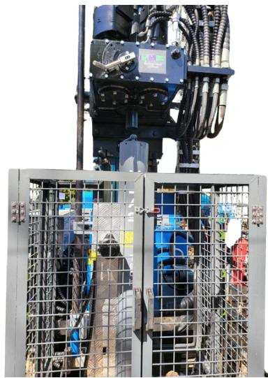
Safety Cover For Drilling and SPT
