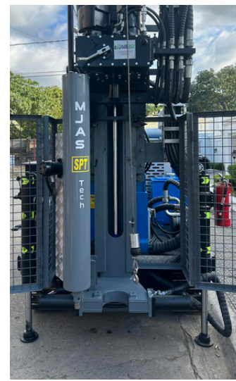
Automatic SPT Hammer
